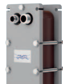
AXP52 is a brazed plate heat exchanger with thin external frames that withstands operating pressures of 130 bar. AXP52 is specially designed to fulfill the need when using CO 2 as refrigerant in subcritical and transcritical applications.
