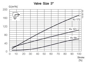
Alfa Laval recommend max. flow velocity in tubing and valves to be 5 m/sec.
