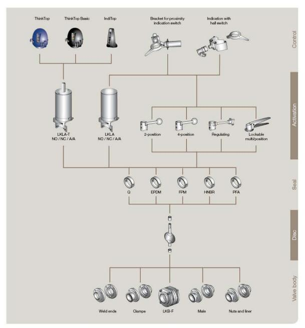
The following selection guide illustrates the many combinations of features and equipment available with LKB butterfly valves. In addition, there are different versions to comply with the full spectrum of worldwide installation standards. As a result, you can always find a configuration to meet any specific requirement.
